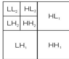
Fig 2 .DWT Subband
