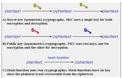
Fig. 2.1: Types of Cryptographic algorithms
