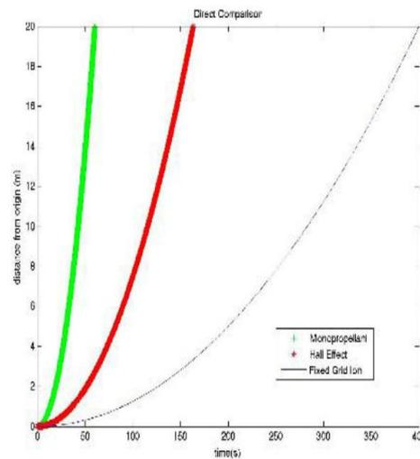
Fig3: Direct comparison of displacement versus time for several thrusters created in Matlab
