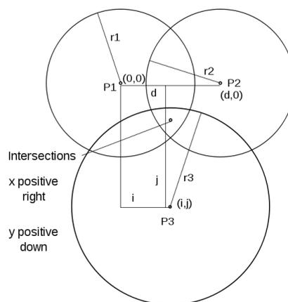
Fig:1: The plane,  $z=0$ , showing the 3 sphere centers, P1, P2, and P3; their x, y coordinates; and the 3 sphere radii,  $r_1$ ,  $r_2$ , and  $r_3$ . The two intersections of the three sphere surfaces are directly in front and directly behind the point designated intersections in the  $z=0$  plane.
