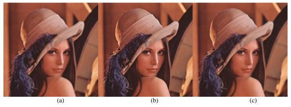
Fig. 4. Comparison of super resolution results for Lena image (with magnification factor 2) using proposed method over other state-of-arts methods: (a) Bicubic interpolation (PSNR: 31.49) (b) Yang et al. [14] (PSNR: 35.03) (c) Proposed scheme (PSNR: 39.20)
