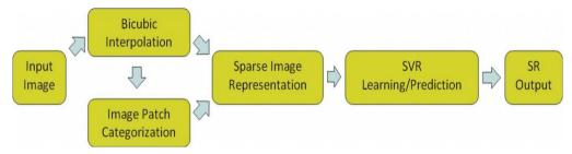
Fig. 3. Flowchart for synthesizing an SR image. This framework does not require the collection of training low and high resolution data in advance
