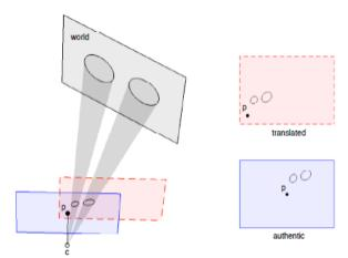
Fig.3 Left: Projection of two eyes (circles) from a world plane (black solid line) onto an image plane (original-blue solid line, translated-red dashed line) with c (camera center) and p (principal point).
