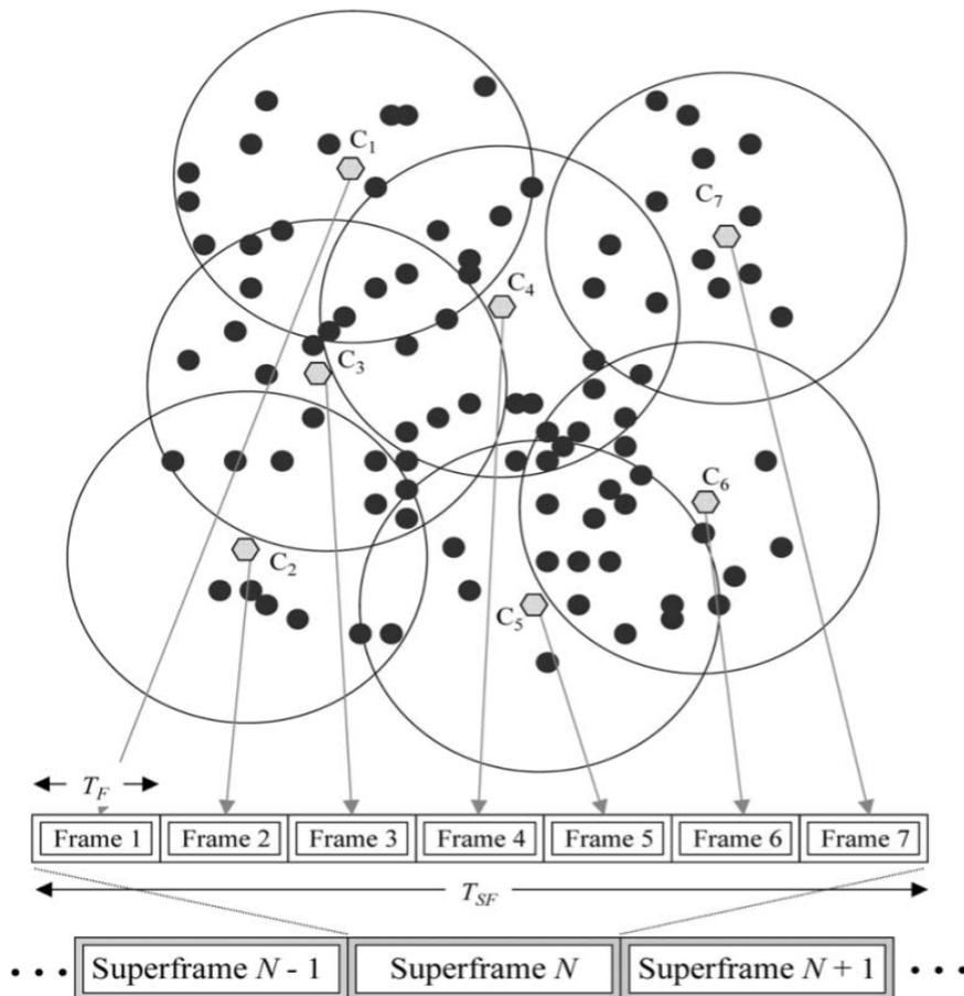
Fig. 1 MH-TRACE clustering and medium access for a portion of an actual distribution of mobile nodes. Nodes C through C are cluster head nodes.
