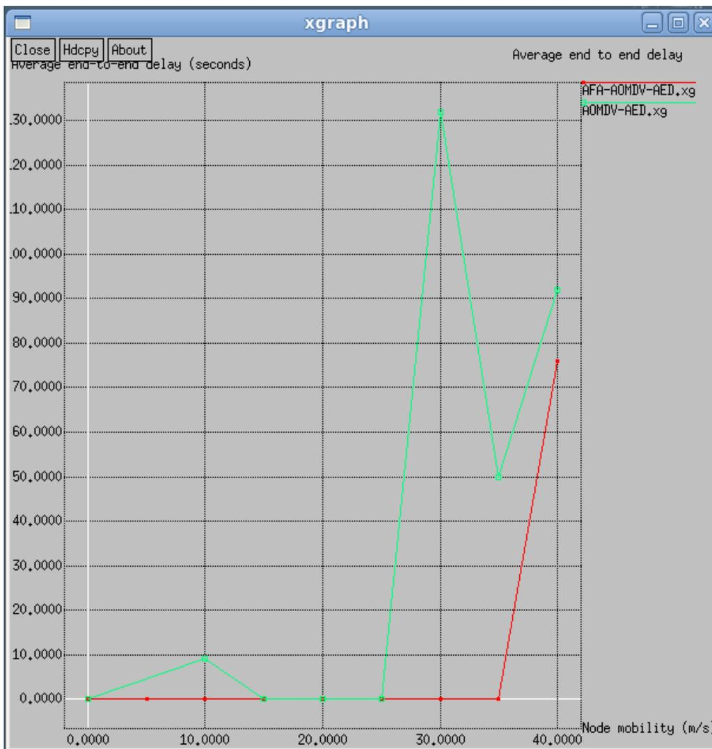
Fig. 2 Comparison of Average end-to-end delay between AFA-AOMDV and AOMDV
