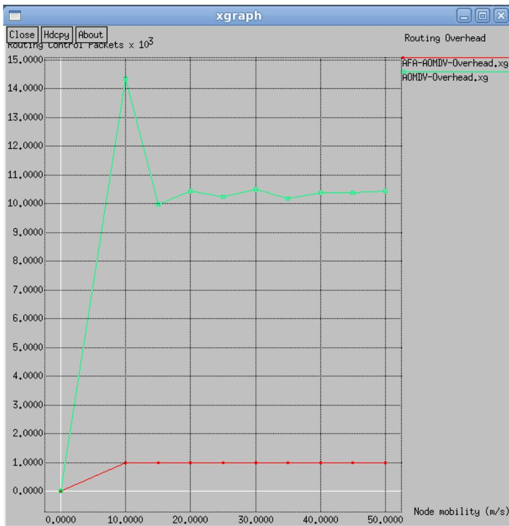
Fig. 3 Comparison of Routing Overhead between AFA-AOMDV and AOMDV
