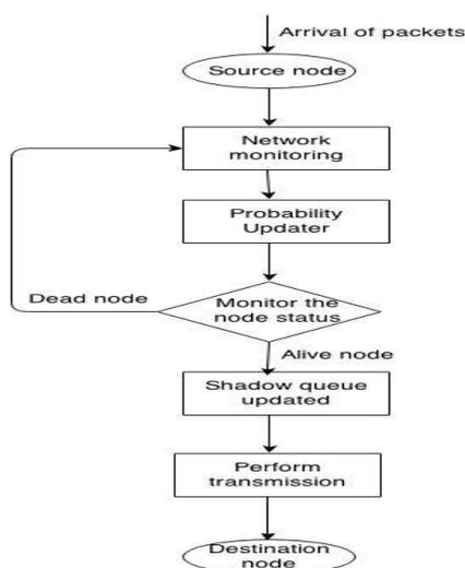
Fig 2 The overall system model
