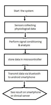
Fig. 3 Flowchart presenting overall system operation
