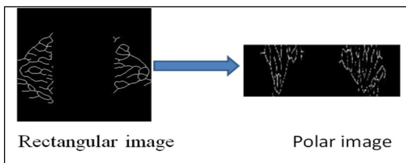
Fig. 9 Conversion of Rectangular to Polar form
