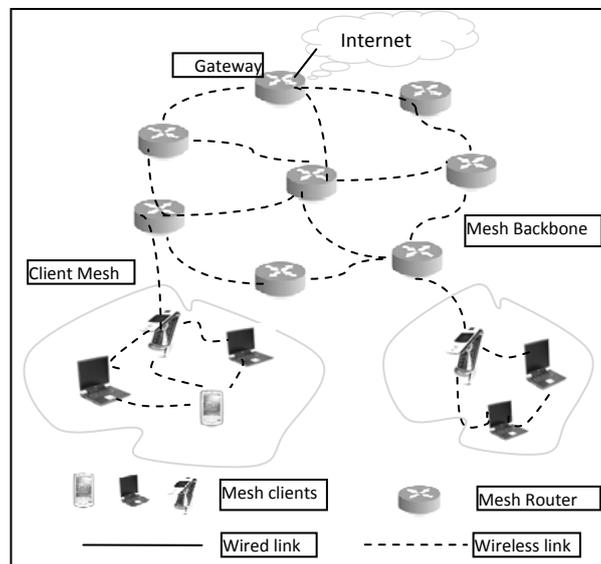
Fig.1 Hybrid Wireless Mesh Network
