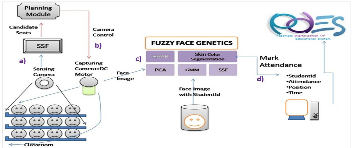
Fig 4: Architecture of the system
