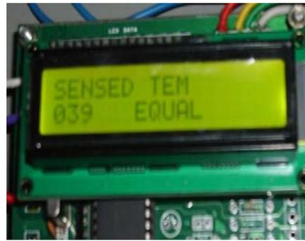
Fig.2. LCD display when the temperature is below 37°C Fig.3. LCD display when the temperature is above 37°C
