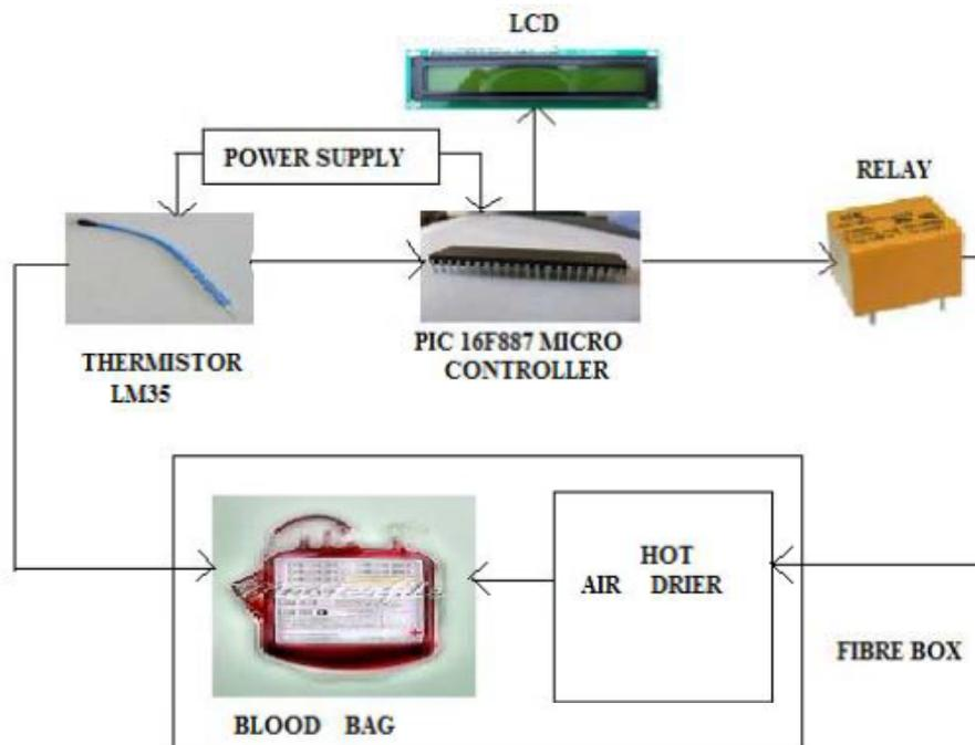
Fig.1. Block diagram of microcontroller based portable paramedic blood warmer for transfusion
