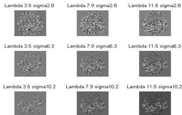
Figure 3: Gabor filter based fingerprint enhancemnet results coreresponding to different values of lambda and sigma
