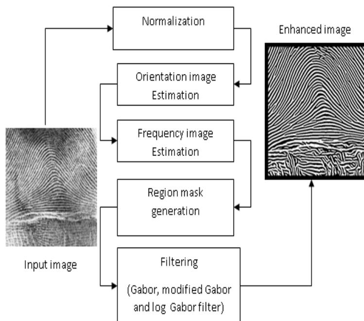
Figure 1: Fingerprint Enhancement algorithm flowchart
