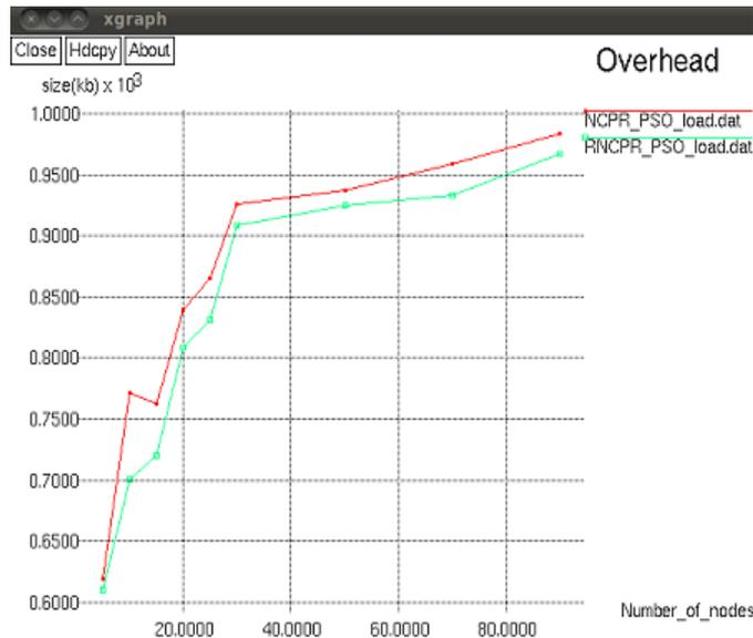
Fig.1. Control Overhead vs number of nodes
