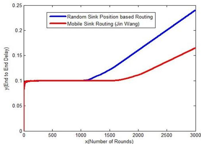
Figure 5: End to End Delay Comparison
