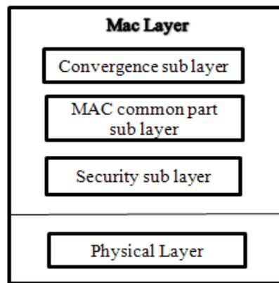
Fig. 1 Structure of IEEE 802.16e standard
