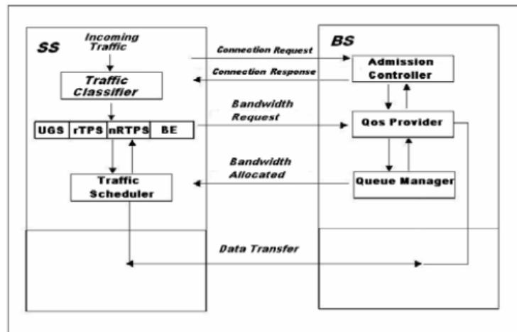
Figure 1 Proposed QoS Model for WiMAX PMP mode
