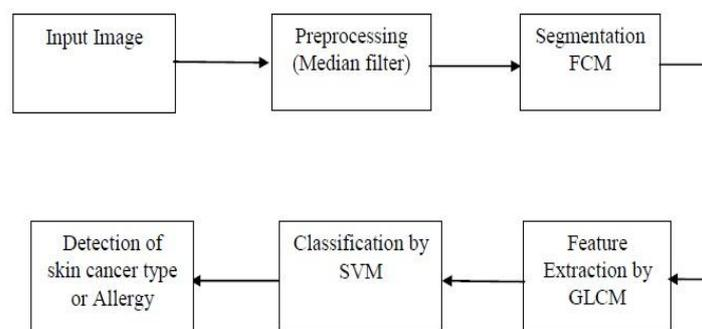
Fig 1.4 Block Diagram
