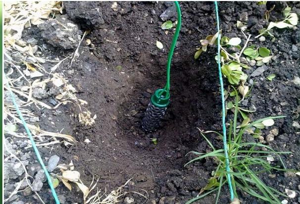
Fig 7. Installation of soil moisture sensor
