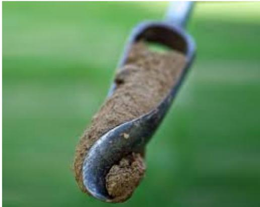
Fig. 6 : Taking soil samples using auger equipment
