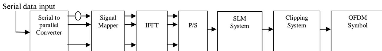
Fig. 6 Block Diagram of SLM-Clipping Hybrid method
