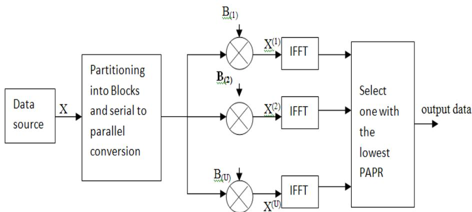
Fig. 5 Block Diagram of SLM technique
