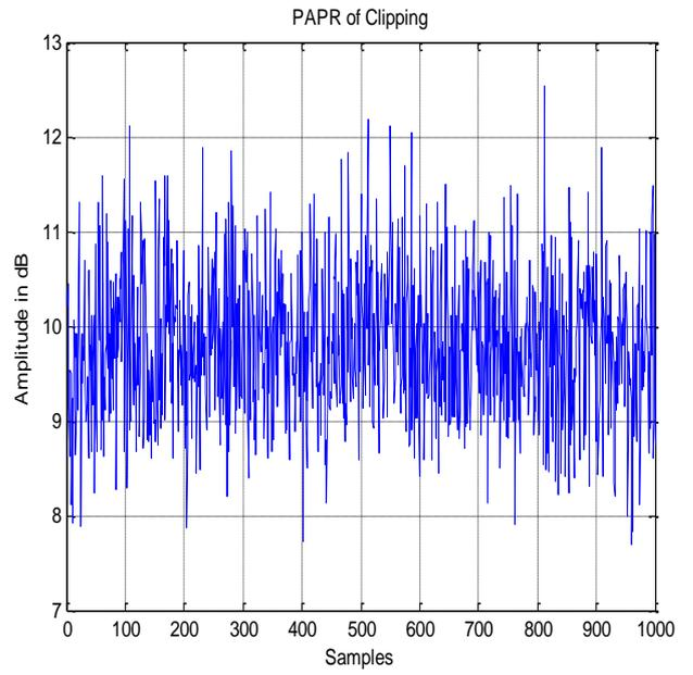
Fig. 8 PAPR of OFDM signal having clipping threshold  $th=0.80$
