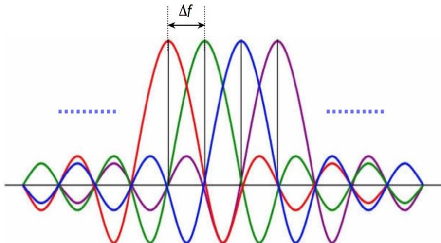
Fig. 1 Orthogonality in 4 subcarriers of an OFDM system
