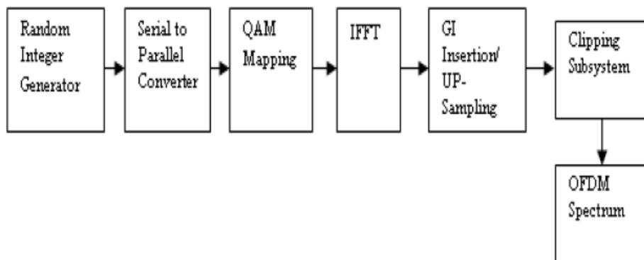
Fig. 4 General Architecture of Clipping
