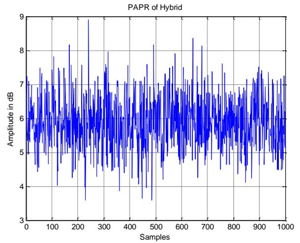
Fig. 10 PAPR of OFDM signal using hybrid method having  $U=4$  &  $th=0.80$
