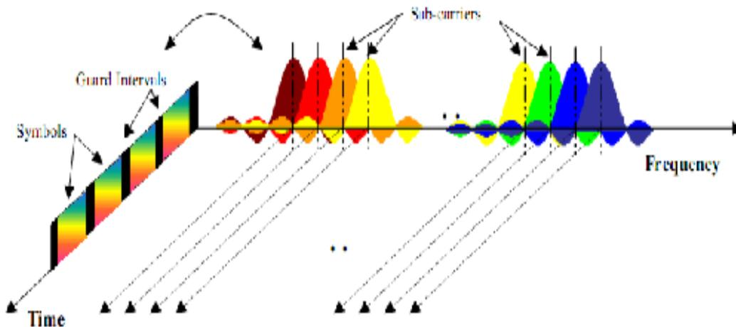
Fig. 2 Frequency & Time domain representation of OFDM signal
