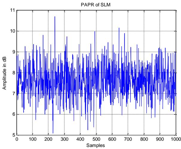
Fig. 9 PAPR of OFDM signal using SLM with  $U=4$
