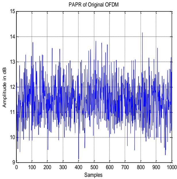
Fig. 7 PAPR of original OFDM signal
