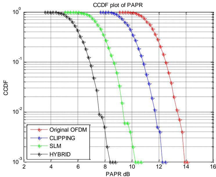
Fig. 11 CCDF Vs PAPR of OFDM signal for  $N=128$
