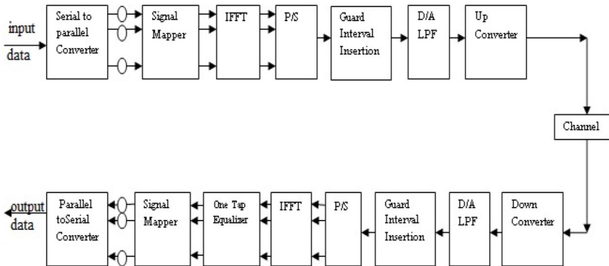
Fig. 3 General Architecture of an OFDM Transceiver system
