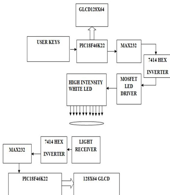
Figure 4: Block diagram of Li-Fi system
