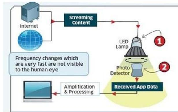
Figure 1: Basic Li-Fi based system
