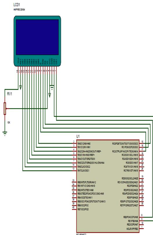
Figure 3: Interfacing GLCD with PIC microcontroller
