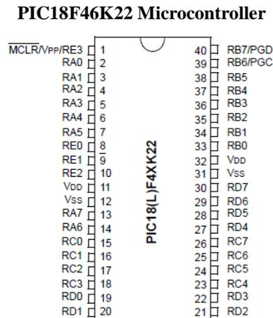
Figure 2: Pin diagram of PIC18F46K22 microcontroller
